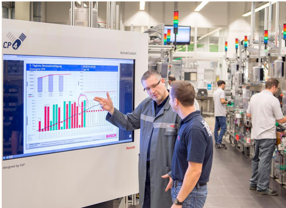
At the Bosch plant in Feuerbach, manufacturing associates use the ActiveCockpit to analyze data from the production process.
